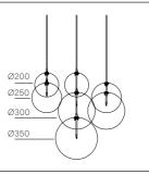
Make sure you match the size of the globe to the size of the tip. Follow the arrangement in the picture where globe diameters are given.
