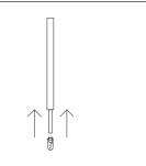
Carefully insert the 71.6W LED G4 bulbs included into the slots at the tip of each arm.
