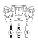
Make all necessary electrical connections. Junction boxes may vary depending on location. The diagram on the left shows the most common markings and manner of connecting the cords.
