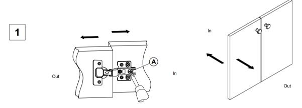
To adjust the door front Left and Right, rotate the adjustment screw (B).
